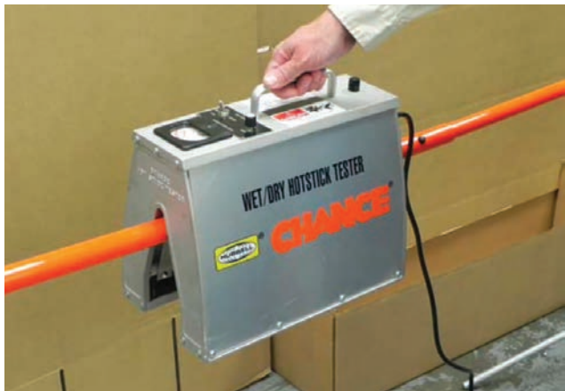
Dielectric testing of hotline equipment. (Hubbell photo)
