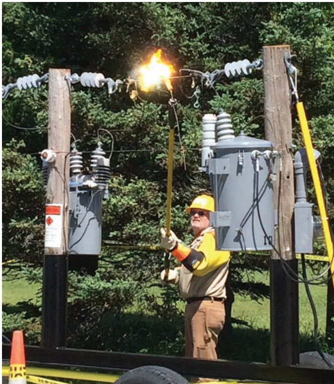
Don Johnson uses our live line demonstrator to cook a hotdog (simulating a finger). Note the insulated "hot stick," rubber gloves, and sleeves that he is wearing.
