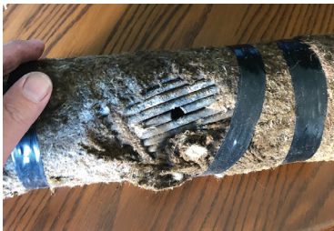
2018 Actual Cable Fault (visit the website for a video of the "thumping" process of locating taken by Hoyt)
